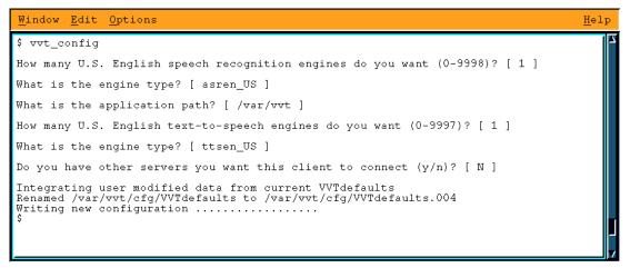
Figure 4-34 Configuration of a speech recognition and text-to-speech engine to support US English
