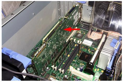
Figure 6-28 Photo of installed Dialogic card
