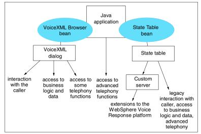
Figure 4-1 Integrating programming models
