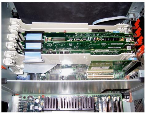
Figure 3-97 Dialogic cards installed with SCBus ribbon
