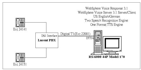
Figure 4-3 Telephony structure for WebSphere Voice Server in ITSO lab
