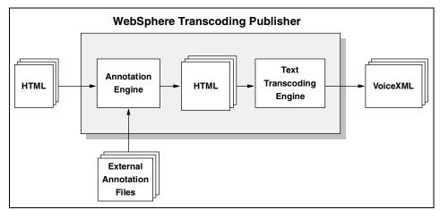
Figure 9-2 Transcoding HTML to VoiceXML
