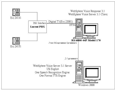
Figure 4-54 Distributed setup of WebSphere Voice Server
