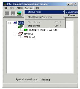
Figure 3-41 Starting up automatically
