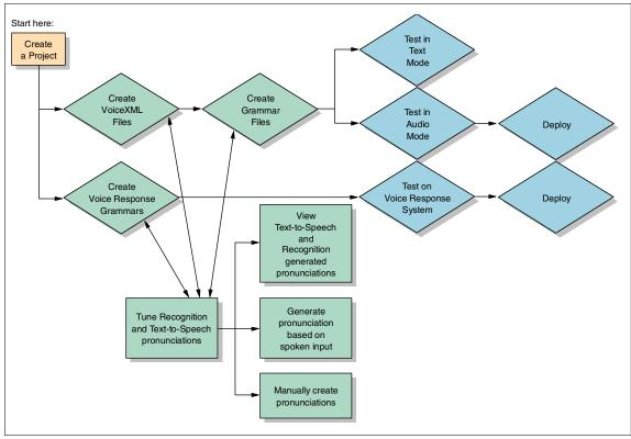
Figure 8-14 Flow of voice application design
