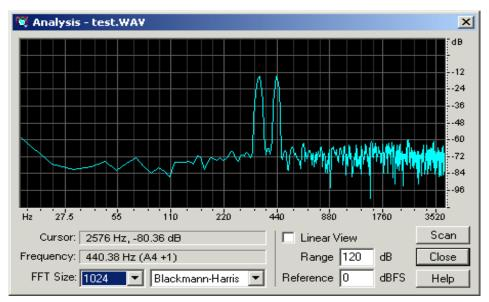
Figure B-14 Non-linear view with FFT of 1024
