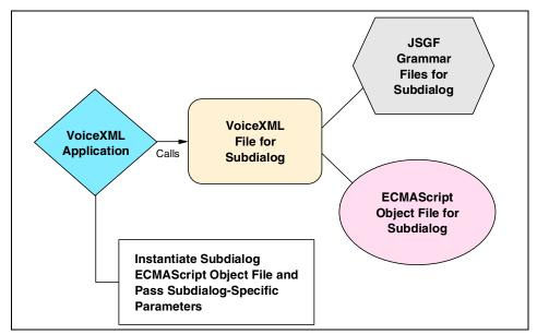
Figure 8-32 Reusable Dialog Components architecture
