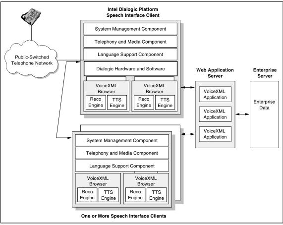
Figure 6-3 Mixed distribution configuration
