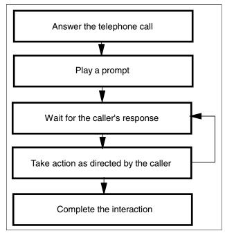
Figure 8-37 Flow chart of a typical call
