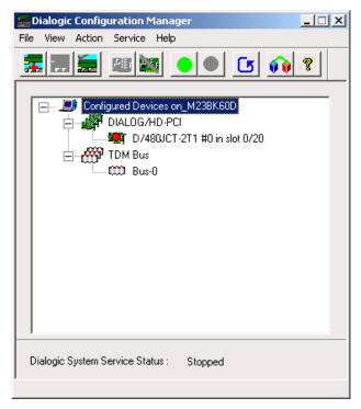
Figure 6-76 DCM window for D/480JCT
